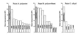
**Figure 4.** Results of gloss measurements (60 °) of the master sample (not exposed to the atmosphere) and specimens exposed for 36-42 months in the different testing stations.
