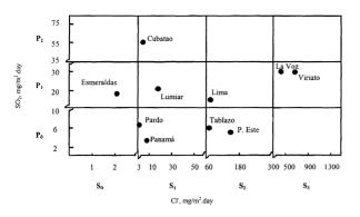
**Figure 1.** Characterization of atmospheres corresponding to the test stations with regard to  $SO_2$  contamination and salinity, according to ISO 9223<sup>[6]</sup>.
