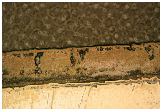
Figure 3. Detail of the artificial magnetite layer of the Iberian falcata, obtained by optical microscopy.
