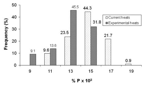
**Figure 4.** Frequency of phosphorus content in the final product (slab) comparing current heats with experimental heats.
