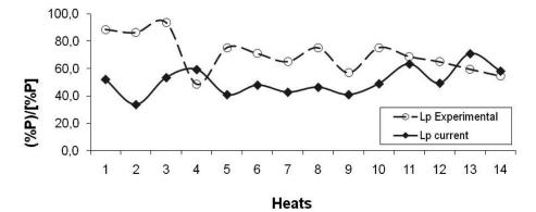
**Figure 3.** Phosphorus partition coefficient in the converter, in the current and experimental heats, where  $Lp = \frac{(\% P)}{[\% P]}$ .
