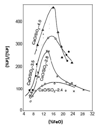
**Figure 1.** Relation between the % FeO in slag, basicity and phosphorus partition  $L_P = \frac{(\% P)}{[\% P]}$ .
