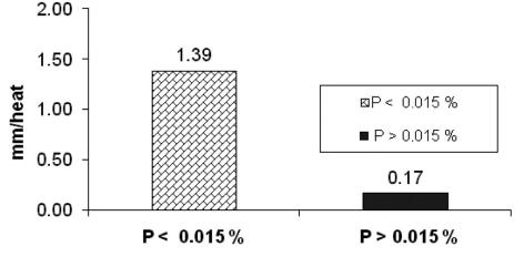
**Figure 5.** Refractory wear rate in converters for current heats ( $P \ge 0.015$ ) and experimental heats ( $P \le 0.015$ ).
