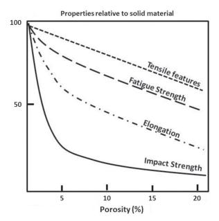
FIGURE 3. Mechanical properties effects due to the level of porosity in PM materials.
