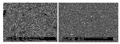
FIGURE 8. High-speed steel manufactured by HIP (left) and metal injection molding (right).
