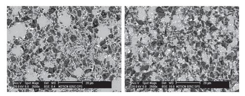
FIGURE 9. SEM microstructures of [M2+0.25 wt% C]/50 vol % TiCN processed (left) pressing at 700 MPa and sintering in vacuum at 1400 °C, 60 minutes, and (rigth) Spark Plasma Sintering (SPS) at 1100 °C and 60 MPa during 10 minutes under vacuum.
