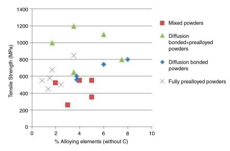
FIGURE 4. Tensile strength for different PM steels (with 0.5% C) manufactured from different kinds of powders and different amounts of alloying elements.
