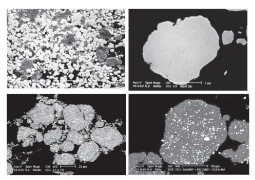
FIGURE 5. Upper-left: mix of aluminum powders (dark) with nickel powders (light). Upper-right: Ni<sub>3</sub>Al intermetallic powder obtained after 20 hours by mechanical alloying. Down-left: composite powders obtained by mechanical alloying: iron reinforced with 25% (vol.) TaC-25 (vol.) NbC. Down-right: 6061 Al alloy reinforced with 5% (vol.) ZrB<sub>2</sub>.
