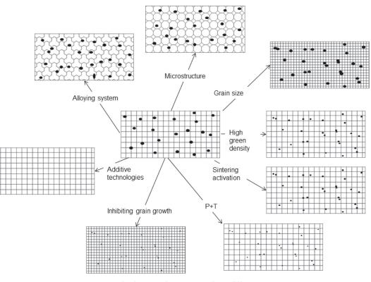
FIGURE 10. Tailoring the microstructure from different PM routes.
