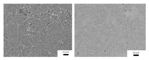
FIGURE 7. YTiAl powder processed by HIP (left) and SPS (right).
