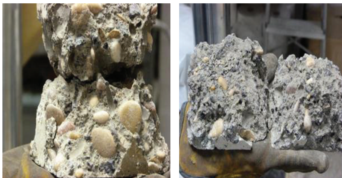
FIGURE 4. Concrete specimens after compression test.
