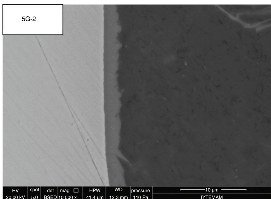
FIGURE 3. Growth of intermetallic layer towards aluminum .
