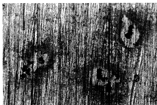
Figure 5. Pitting corrosion attack by sulphate-reducing bacteria on stainless steel Type UNS S42000 annealed (50x) (Printing reproduction at 53 %).
