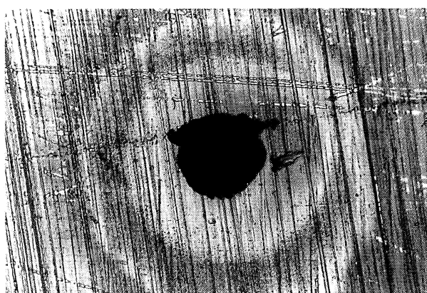
Figure 10. Pitting corrosion on stainless steel Type UNS S42000 quenched and tempered after an electrochemical test using Electrolyte B (400x) (Printing reproduction at 53 %).
