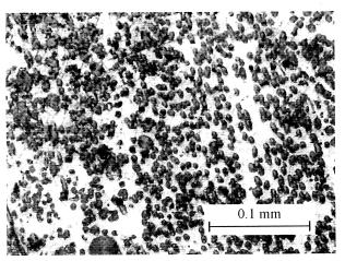
Figure 2. Metallographic image of Al-VGCF
