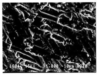
Figure 15. SEM image of the tribofilm formed on the pin of Al-exPAN
