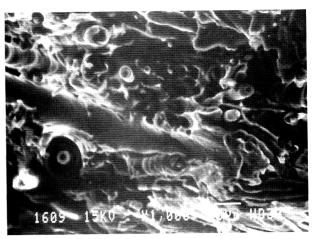
Figure 6. Three-point bending test of Al 5% Si (UTS<sub>max</sub>=282.1 MPa), and its composite with exPAN (UTS<sub>max</sub>=331.4 MPa)
