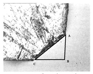
Figure 11. Measurement of wear with image analysis
