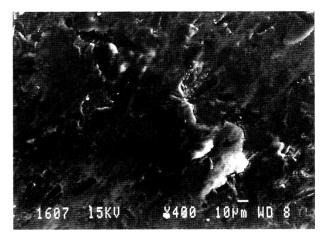
**Figure 13.** SEM image of the tribofilm and matrix delamination on the pin of Al-VGCF
