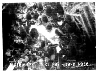
Figure 5. SEM image of Al-exPAN fracture
