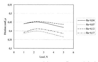
Figure 10. Variation of friction coefficient with load, v=0.30 m/s
