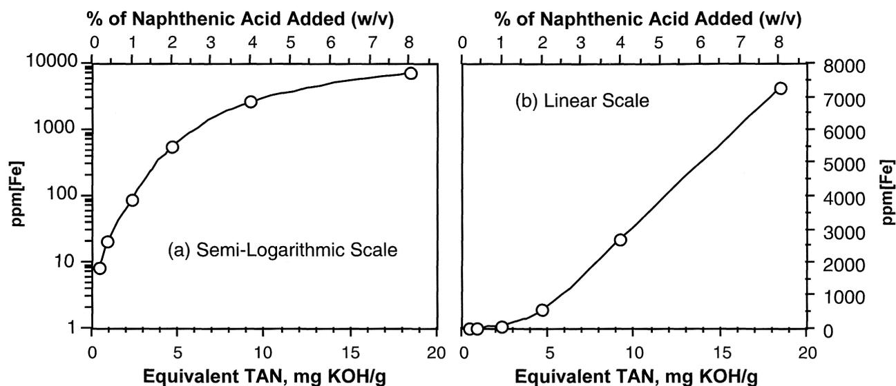
**Figure 1.** Maximum amount of iron dissolved as a function of the naphthenic acid added into white oil, after performing the Fe powder test. (a) Semi-Logarithmic scale and (b) Linear scale.
