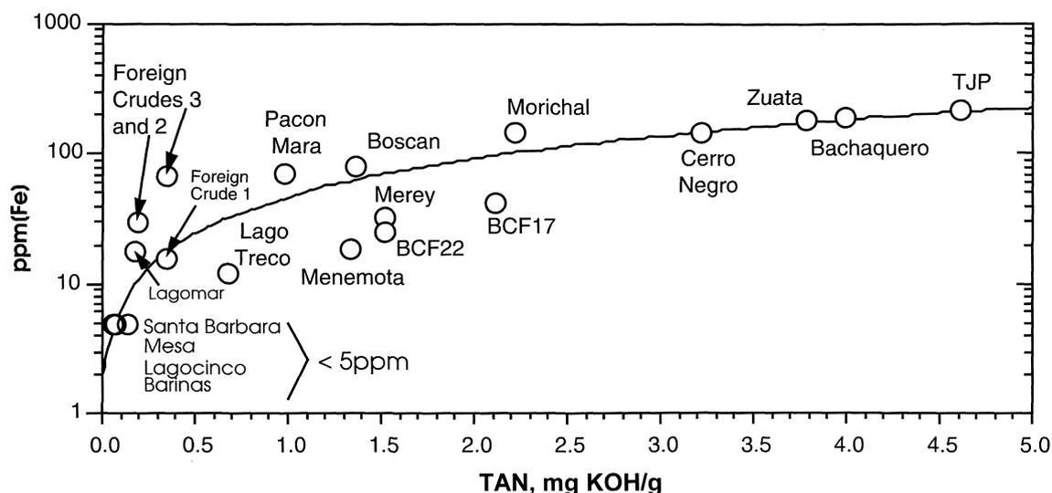
**Figure 3.** Correlation between the maximum amount of iron dissolved, as determined in the Fe powder test, and the TAN for real crude oil samples.
