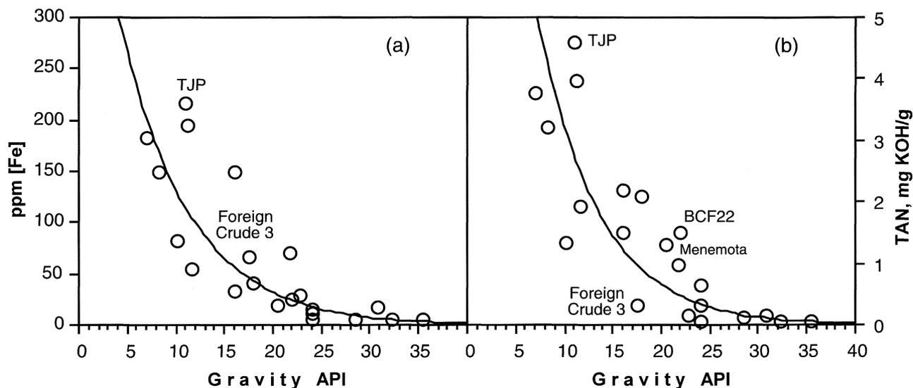
**Figure 4.** Correlation between the maximum amount of iron dissolved, as determined in the Fe powder test, TAN, and the API gravity of real crude oil samples.
