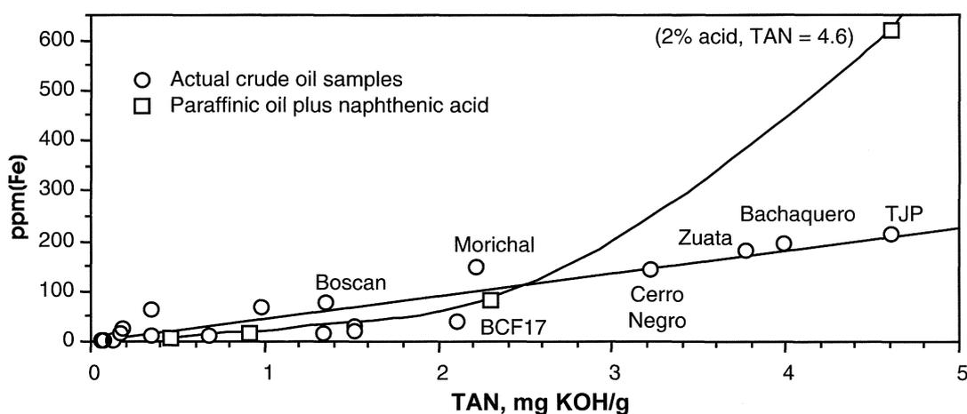
**Figure 2.** Comparison between the results obtained with the Fe powder test for real crude oil samples and for the mixture of paraffinic with addition of commercially available low-sulfur naphthenic acid.
