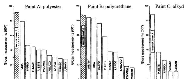
**Figure 4.** Results of gloss measurements (60 °) of the master sample (not exposed to the atmosphere) and specimens exposed for 36-42 months in the different testing stations.
