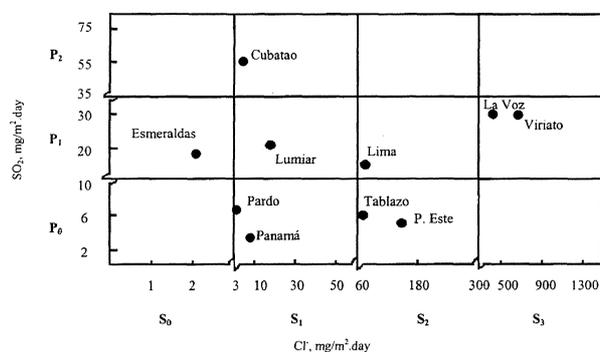
**Figure 1.** Characterization of atmospheres corresponding to the test stations with regard to SO<sub>2</sub> contamination and salinity, according to ISO 9223<sup>[6]</sup>.
