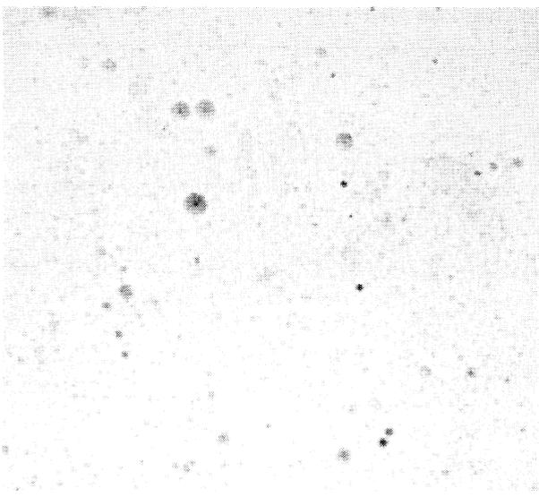
**Figure 3.** Presence of fungi on the surface of paint C exposed in Lumiar atmosphere.
