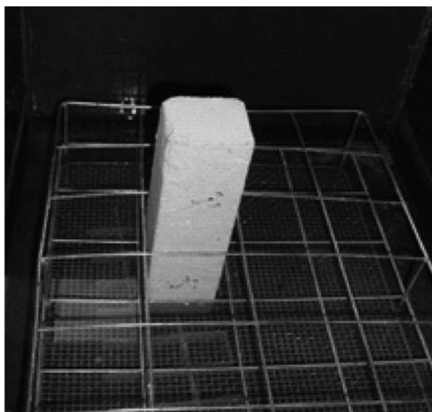
Figure 1. Positioning of sample in chamber for capillary absorption test.
