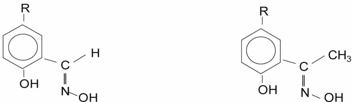
**Figure 4.** Basic structures of aldoximes (left) and ketoximes (right).
