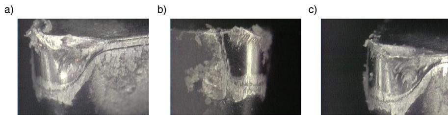
FIGURE 3. Tool wear in coated WC tool with a neutral rake angle ( $0^\circ$ ) at  $200 \text{ m min}^{-1}$ .
