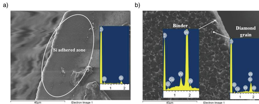
FIGURE 6. SEM image of the MCD surface : (a) where it can be seen a shaded area that contains silicon; (b) the fine grain PCD surface.
