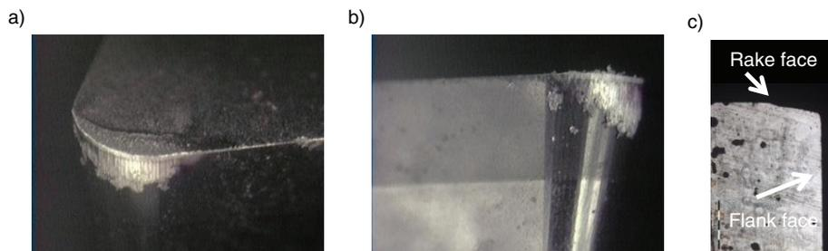
FIGURE 4. Tool wear in PCD tool with a positive rake angle ( $+6^\circ$ ) at  $500 \text{ m min}^{-1}$ .
