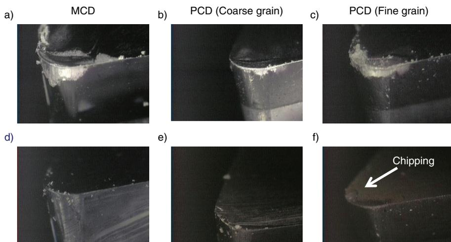
FIGURE 5. Top row, tools after machining. Bottom row, tools after chemical cleaning to remove the BUE.  $400 \text{ m min}^{-1}$ . Rake angle  $0^\circ$ .
