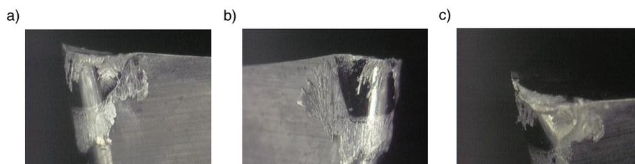
FIGURE 2. Tool wear in uncoated WC tool with a positive rake angle ( $+30^{\circ}$ ) at  $200 \text{ m min}^{-1}$ .
