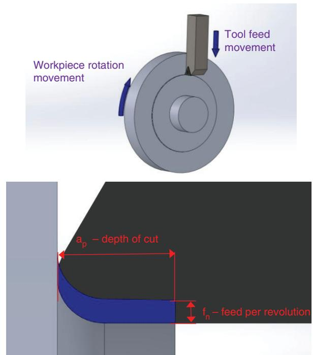
FIGURE 1. Scheme of the machining operation.
