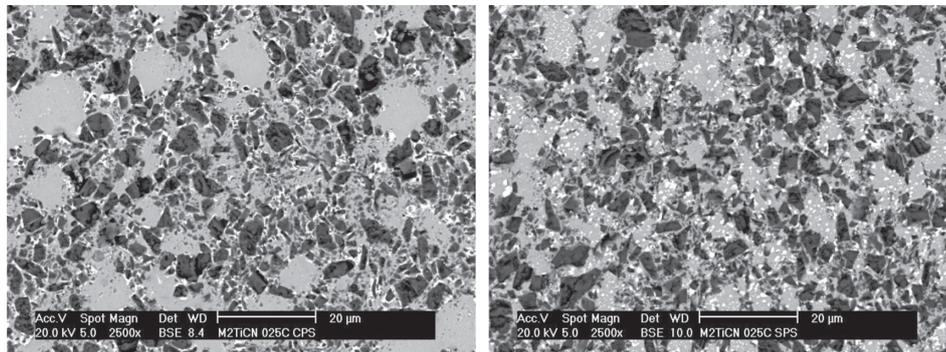
FIGURE 9. SEM microstructures of [M2 + 0.25 wt% C]/50 vol % TiCN processed (left) pressing at 700 MPa and sintering in vacuum at 1400 °C, 60 minutes, and (right) Spark Plasma Sintering (SPS) at 1100 °C and 60 MPa during 10 minutes under vacuum.
