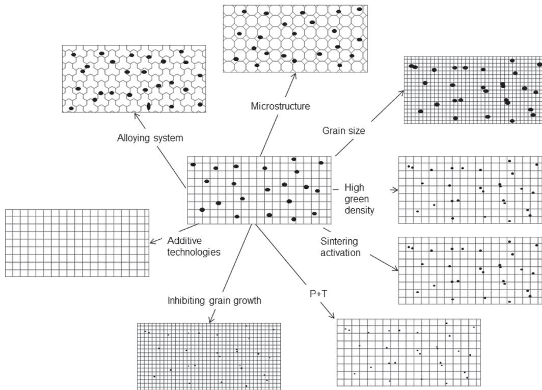
FIGURE 10. Tailoring the microstructure from different PM routes.
