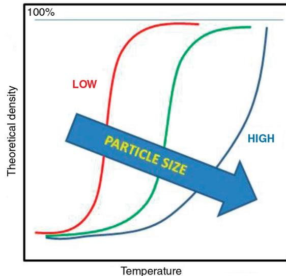
FIGURE 6. Influence of particle size on densification in a sintering process.
