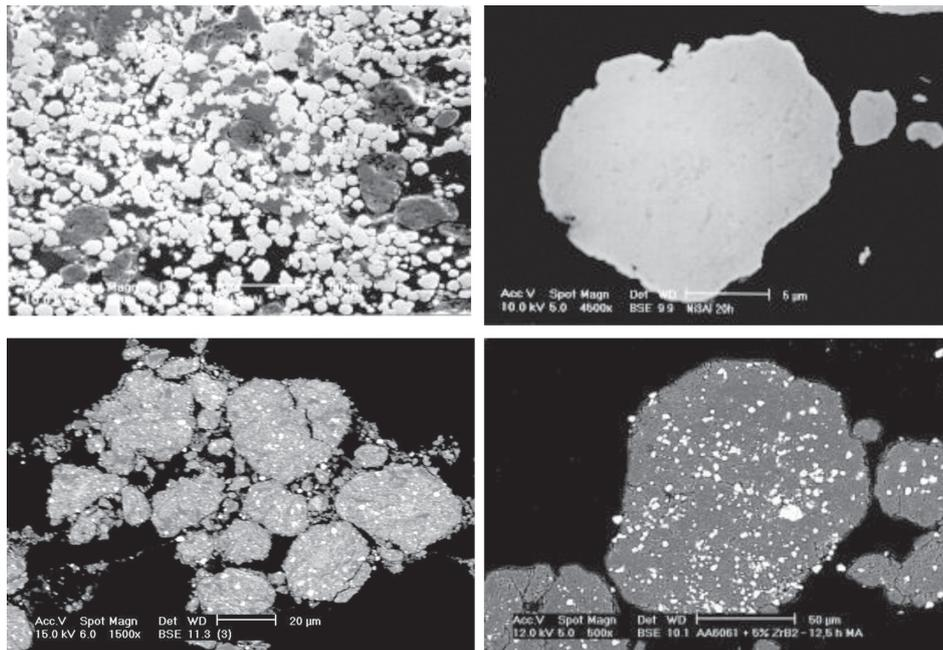
FIGURE 5. Upper-left: mix of aluminum powders (dark) with nickel powders (light). Upper-right:  $\text{Ni}_3\text{Al}$  intermetallic powder obtained after 20 hours by mechanical alloying. Down-left: composite powders obtained by mechanical alloying: iron reinforced with 25% (vol.) TaC-25 (vol.) NbC. Down-right: 6061 Al alloy reinforced with 5% (vol.)  $\text{ZrB}_2$ .
