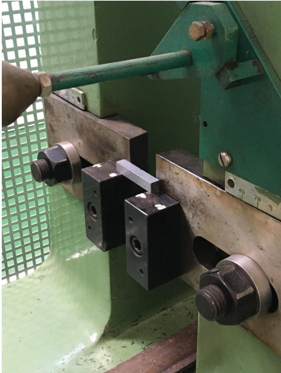
FIGURE 3. Sample used to test using Charpy impact.
