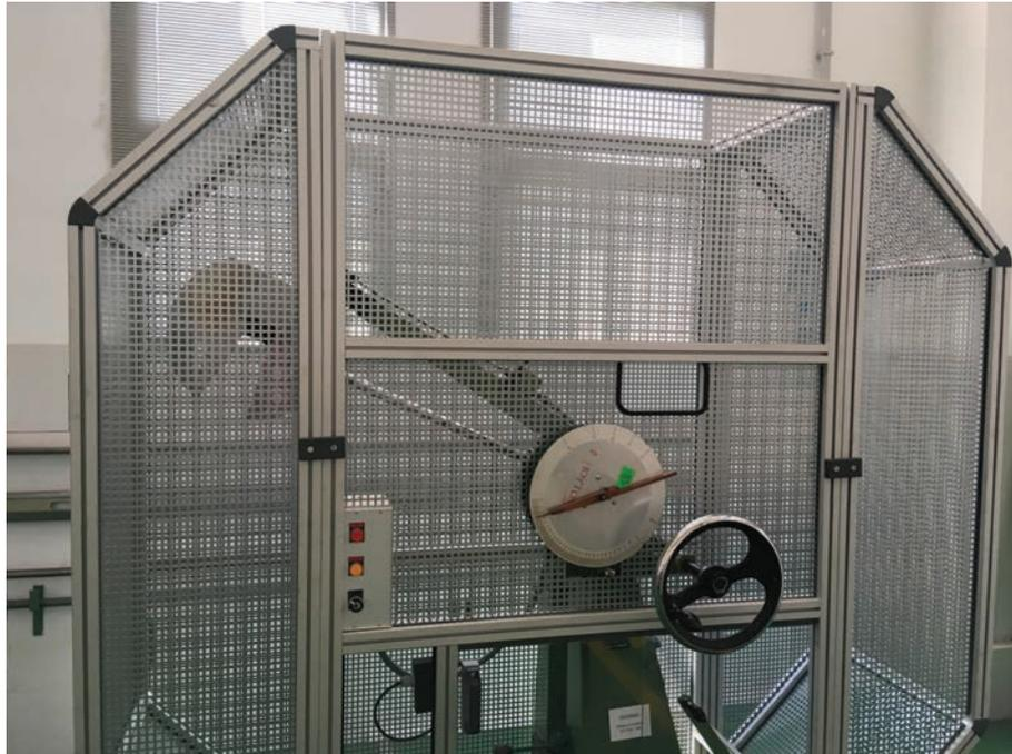
FIGURE 2. Photo of the Charpy pendulum used to teach students.
