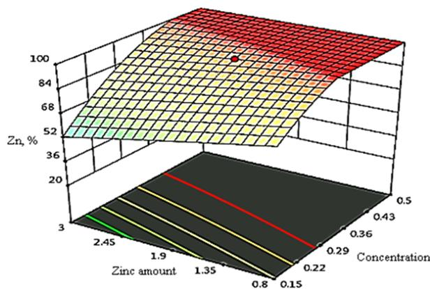
FIGURE 3. The interactive effect of the concentration of nitric acid and the amount of zinc on the dissolution yield.
