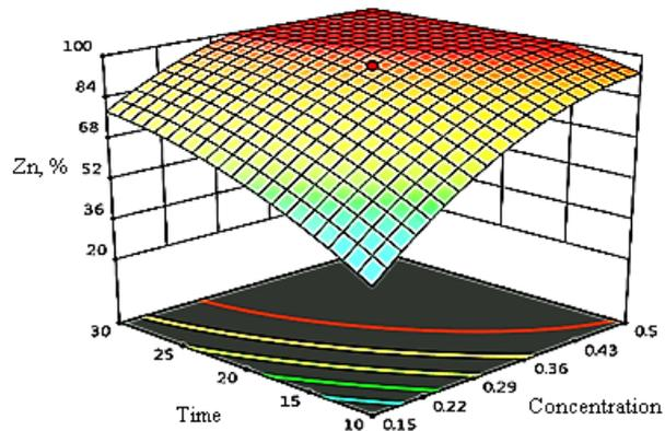
FIGURE 4. The interactive effect of the concentration of nitric acid and the reaction time on the dissolution yield.
