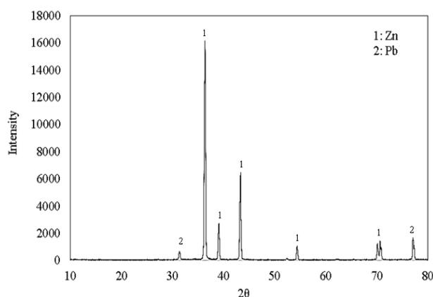
FIGURE 1. XRD analysis of the cleaned zinc plate obtained from waste zinc carbon battery.
