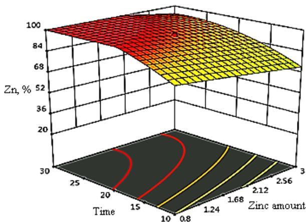
FIGURE 5. The interactive effect of the amount of zinc and the reaction time on the dissolution yield.
