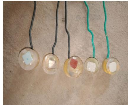
FIGURE 2. Linear Polarization Resistance (LPR) Specimen.
