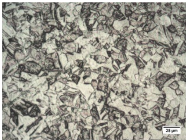
FIGURE 4. Micrograph of the bronze and manganese alloy (filler material).
