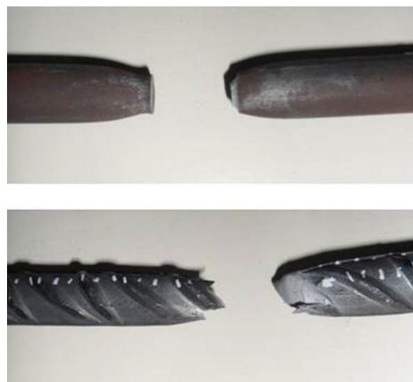
Figure 10. Type of failure for smooth bars (top) and ribbed bars (bottom).
