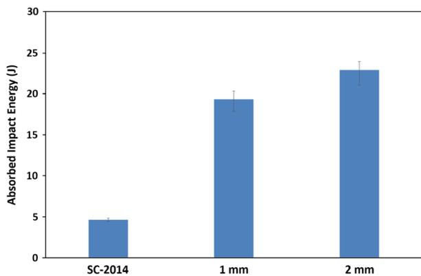
FIGURE 8. Total absorbed impact energies of the specimens.
