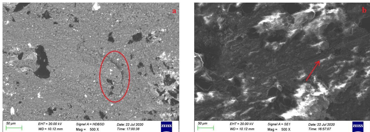
FIGURE 12. SEM image of the worn 2-mm thick composite surface a) plastic deformation of the metal matrix (highlighted by an ellipse), b) groove of an abrasive particle (pinpointed by a red arrow).
