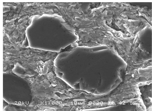
FIGURE 4. SEM image showing the boron carbide particle and the surrounding aluminum matrix of 1-mm thick specimen.
