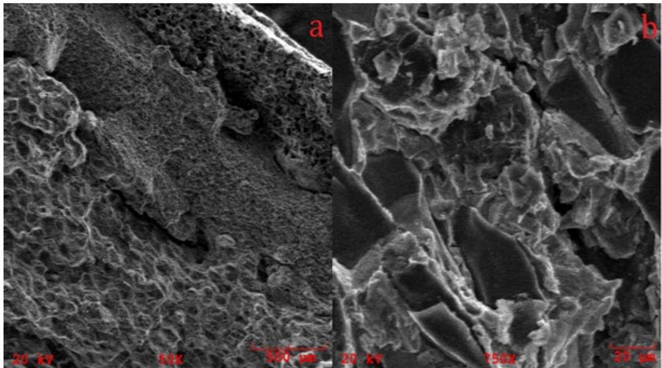
FIGURE 7. SEM images of the fracture characteristics of a) aluminium matrix and b) interface (red arrow) of the tensile specimen of 1-mm thick.
