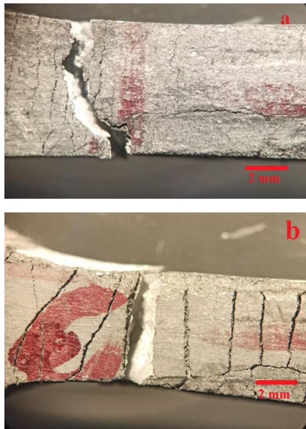
FIGURE 6. Cracks formed perpendicular to the tensile direction in the composite layer a) 1 mm, b) 2 mm.
