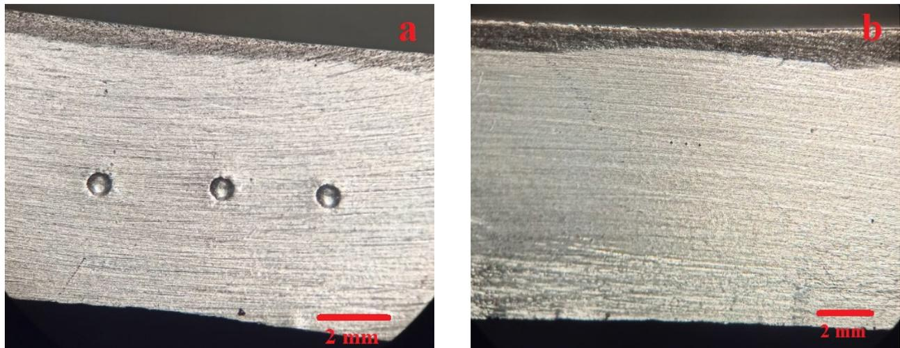
FIGURE 2. Stereomicroscope images of the cross-sections of the composite materials a) 1 mm, b) 2 mm.
