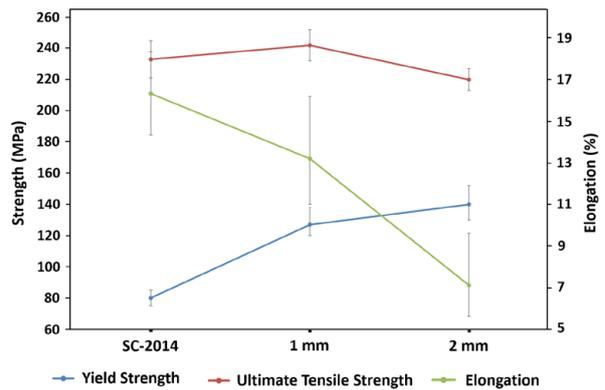
FIGURE 5. Tensile test properties of the composites compared to the AA2014 aluminum wrought alloy.
