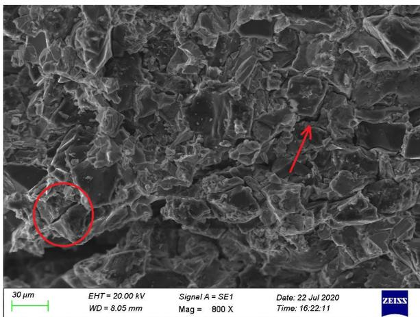
FIGURE 9. The fracture surfaces of the impact test of the 1-mm thick specimen (Cracks have been pinpointed with a red circle and a red arrow).
