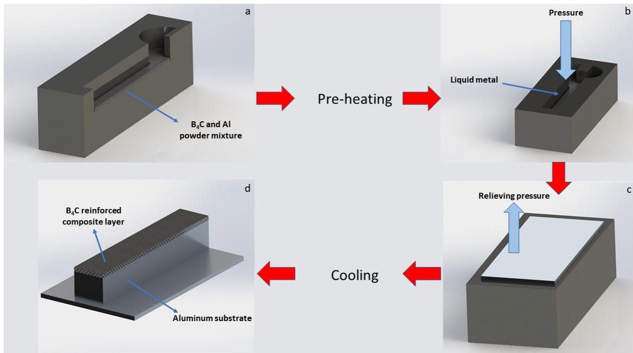
FIGURE 1. MMC production steps with squeeze casting.
