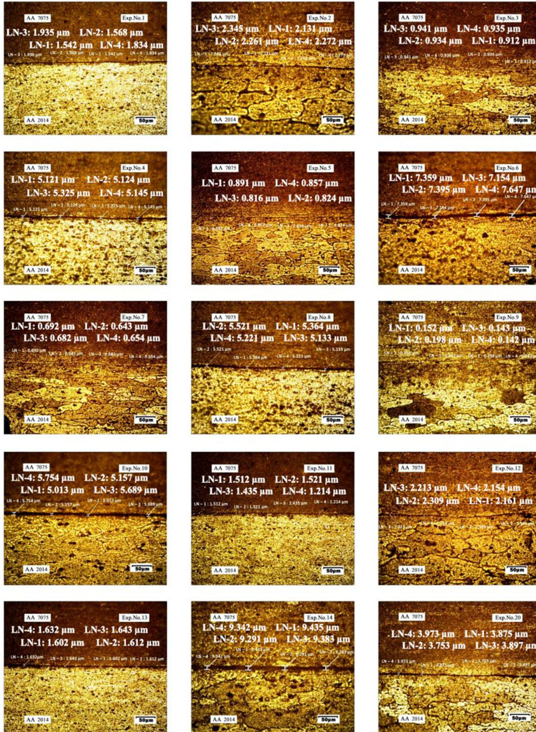
Figure. 3. Optical images of the microstructures of the joints showing the interface thickness variation for different bonding conditions.
