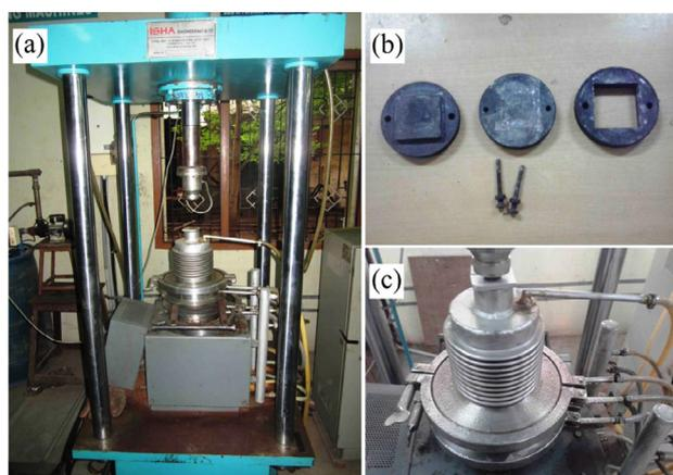
FIGURE 1. Experimental Setup, (a) Diffusion bonding machine; (b) 316L Stainless steel die; (c) Vacuum furnace.
