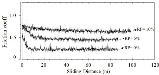
FIGURE 2. Friction coefficient variation throughout the tests for the sample samples.
