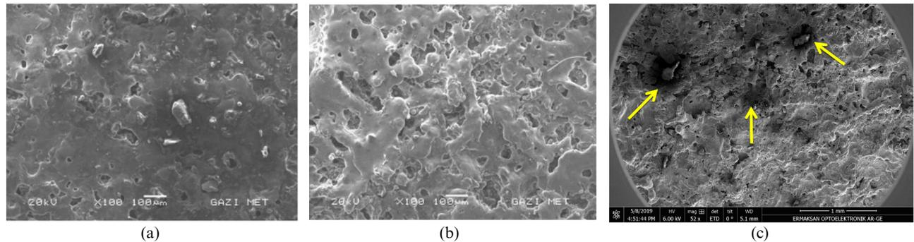
FIGURE 6. Samples machined at RP = 10%, = 8 A; (a) PM/EDM (b) EDM, (c) B<sub>4</sub>C lumps.
