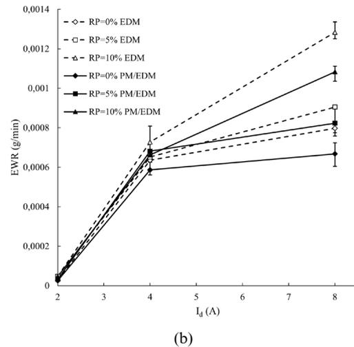
FIGURE 5. Effect of  $I_d$  on a) the WRR, and b) the EWR for various RP values and machining types.
