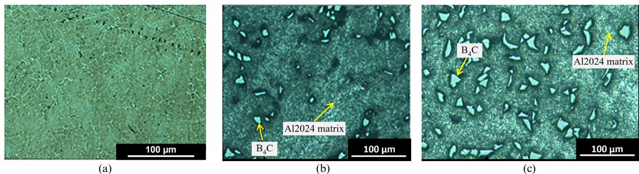
FIGURE 1. The microstructure images: (a) RP = 0%, (b) RP = 5%, (c) RP = 10%.
