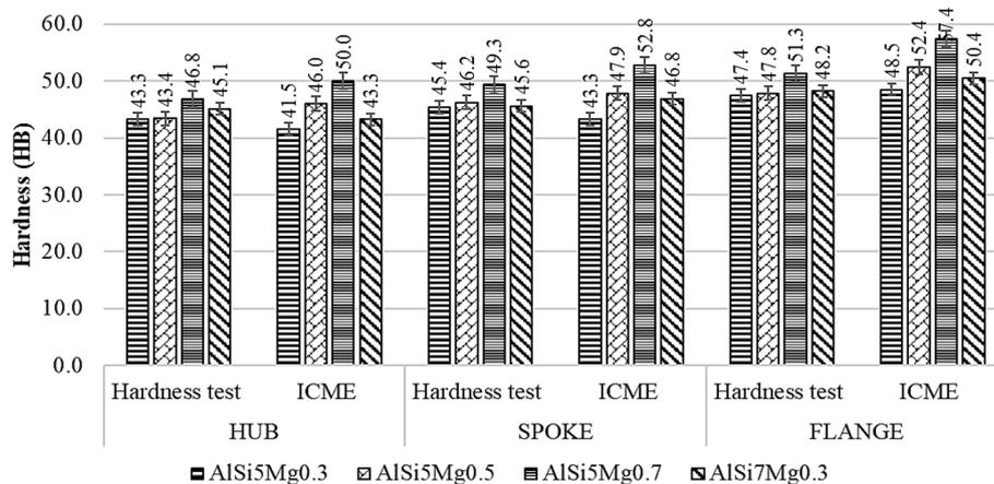
**Figure 11.** Comparative plot of hardness values for the hub, spoke and flange calculated with the ICME and obtained from the tensile test results
