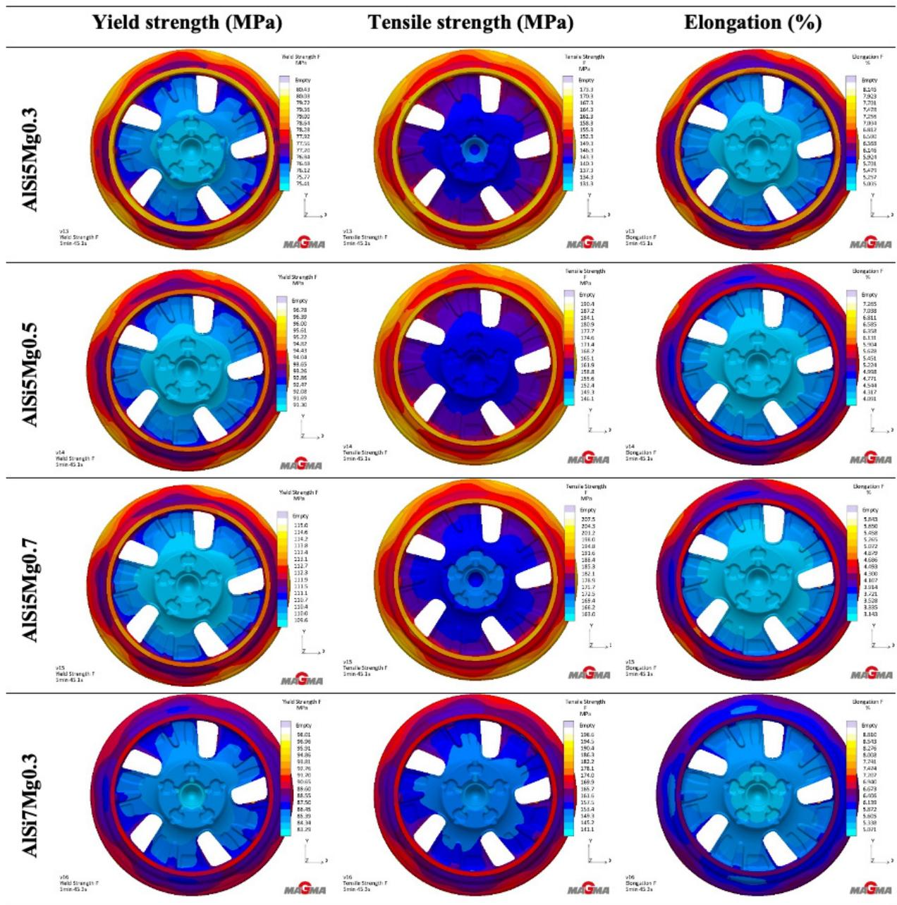
FIGURE 5. MagmaSoft analysis results of the mechanical properties in wheels depending on chemical composition of the alloys.
