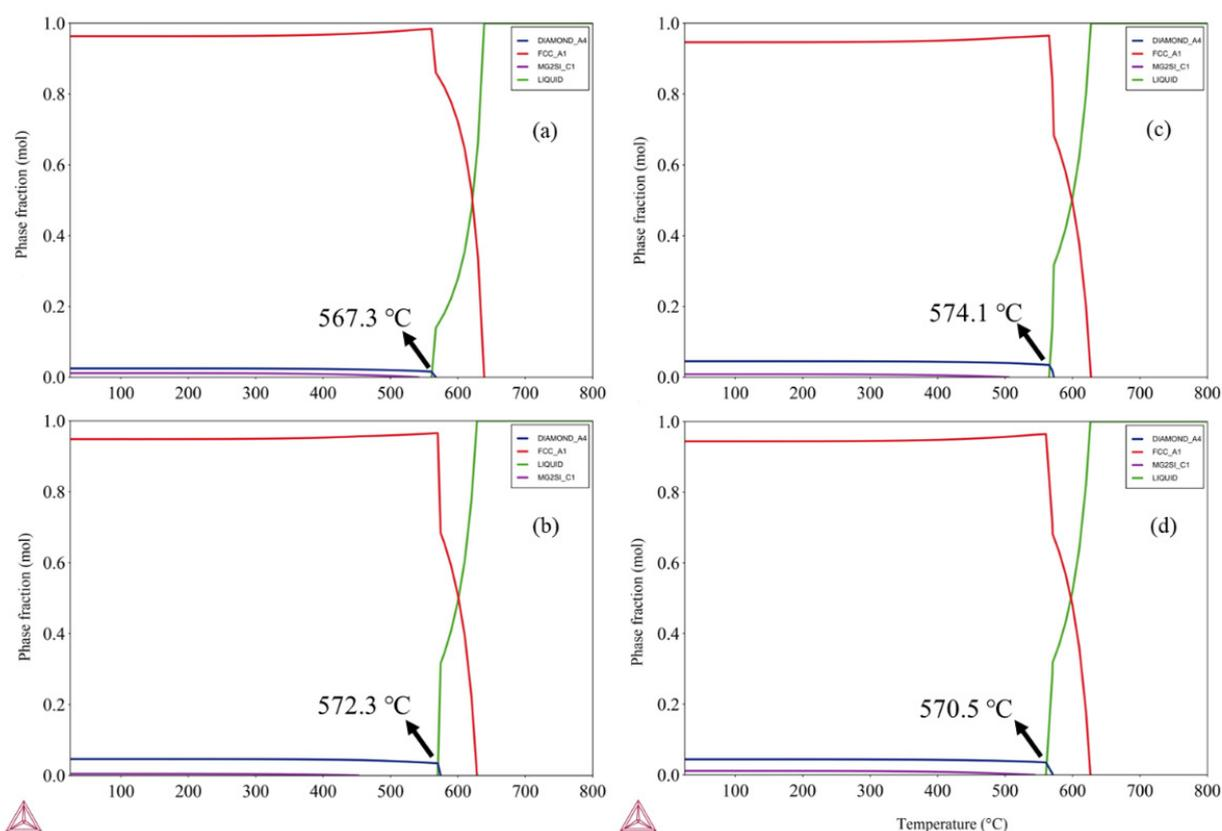
FIGURE 2. The graphs phase fractions changes of alloys with temperature under equilibrium conditions: (a) AlSi5Mg0.3, (b) AlSi5Mg0.5, (c) AlSi5Mg0.7, (d) AlSi7Mg0.3 obtained with CME-ThermoCalc. The marked points represent the eutectic transformation temperatures.
