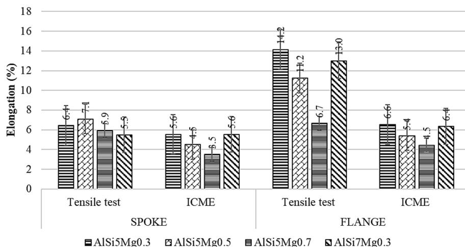
Figure 10. Comparative plot of elongation values for the spoke and flange calculated with the ICME and obtained from tensile test results
