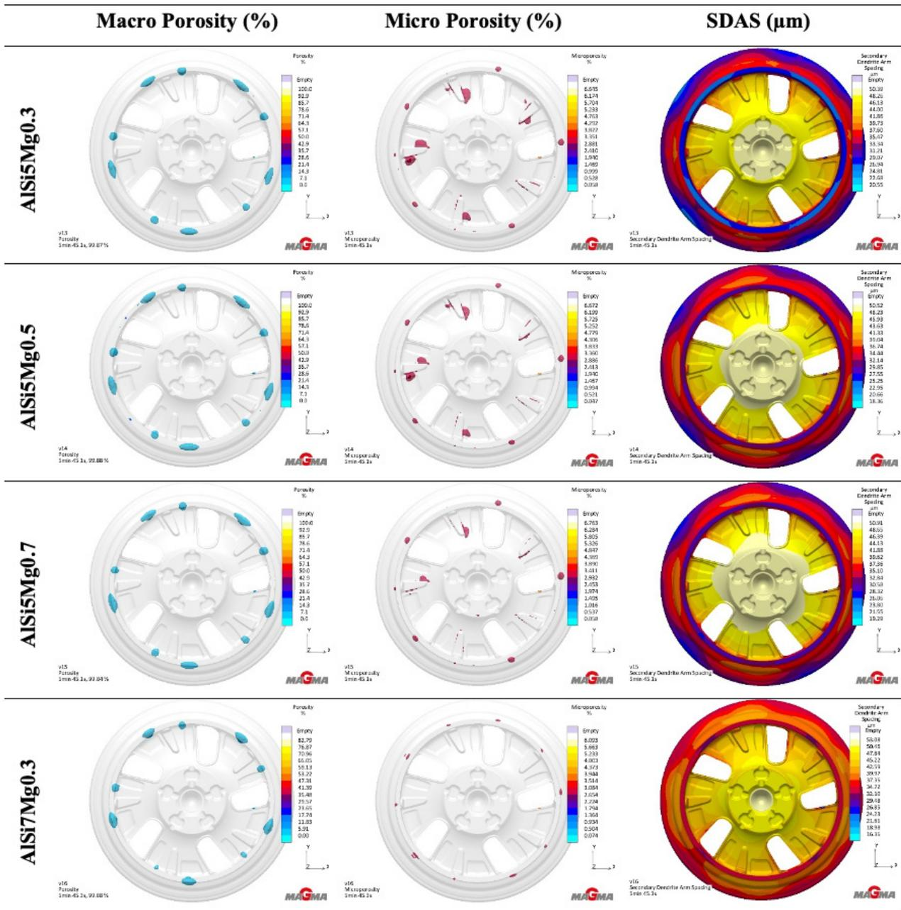
FIGURE 4. MagmaSoft analysis results of the microstructural properties in wheels depending on chemical composition of the alloys.
