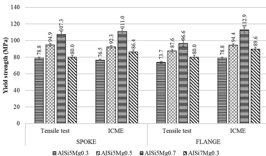
FIGURE 9. Comparative plot of yield strength values for the spoke and flange calculated with the ICME and obtained from the tensile test results.
