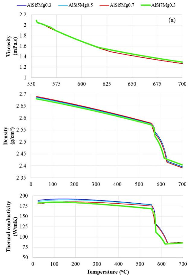
FIGURE 1. Temperature dependent graphs of (a) liquid viscosity, (b) density and (c) thermal conductivity values of alloys calculated by CME-JMatPro
