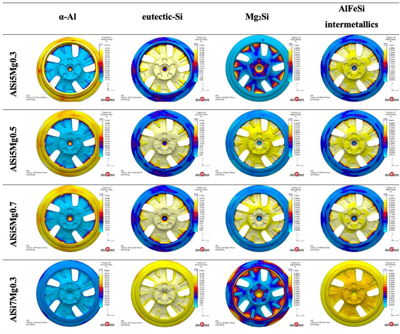
FIGURE 3. Phase distribution in wheels depending on alloy composition.
