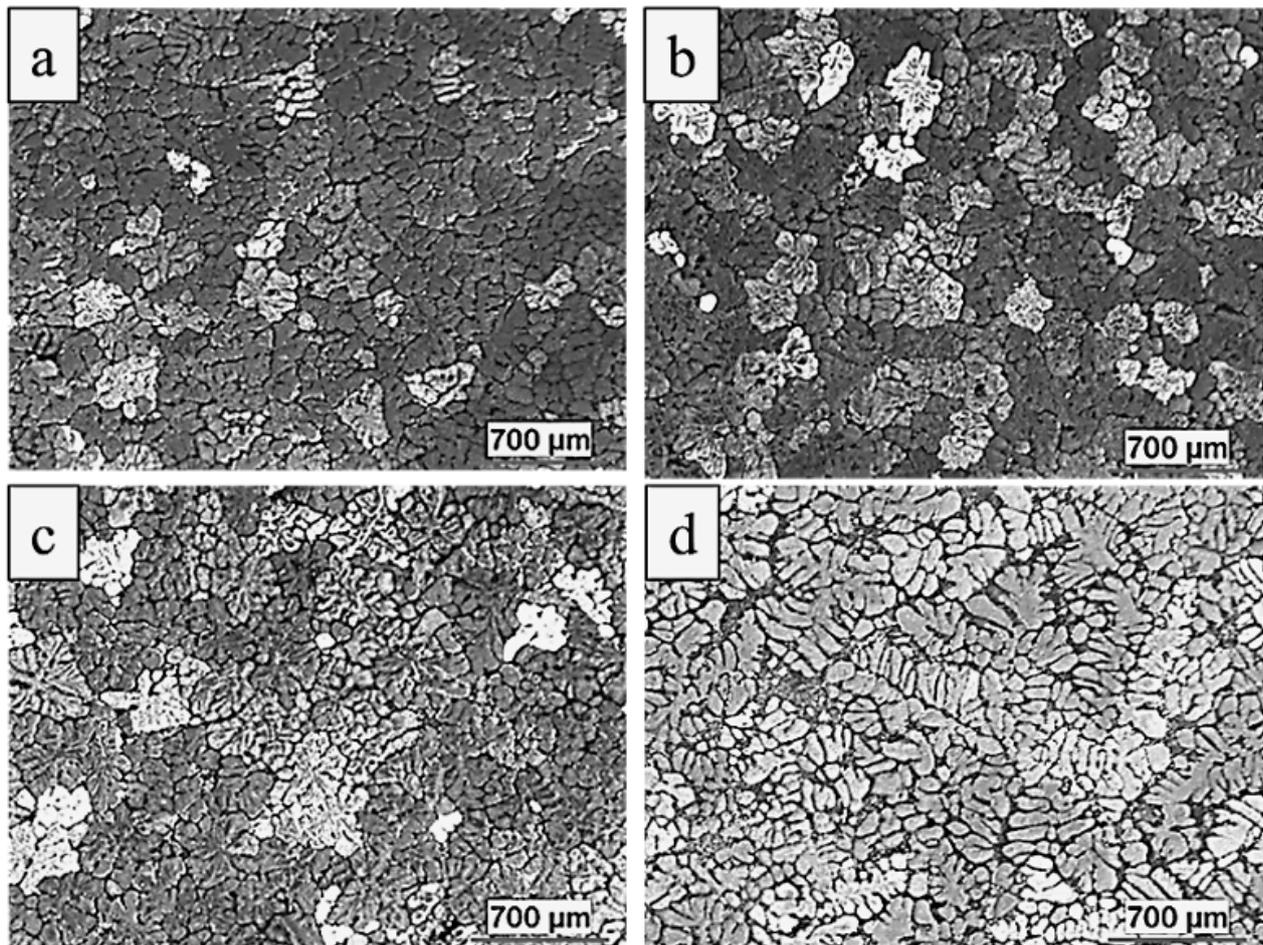
FIGURE 6. Stereo microscope images from the hub of the samples (30x), a) AlSi5Mg0.3, b) AlSi5Mg0.5, c) AlSi5Mg0.7, d) AlSi7Mg0.3.
