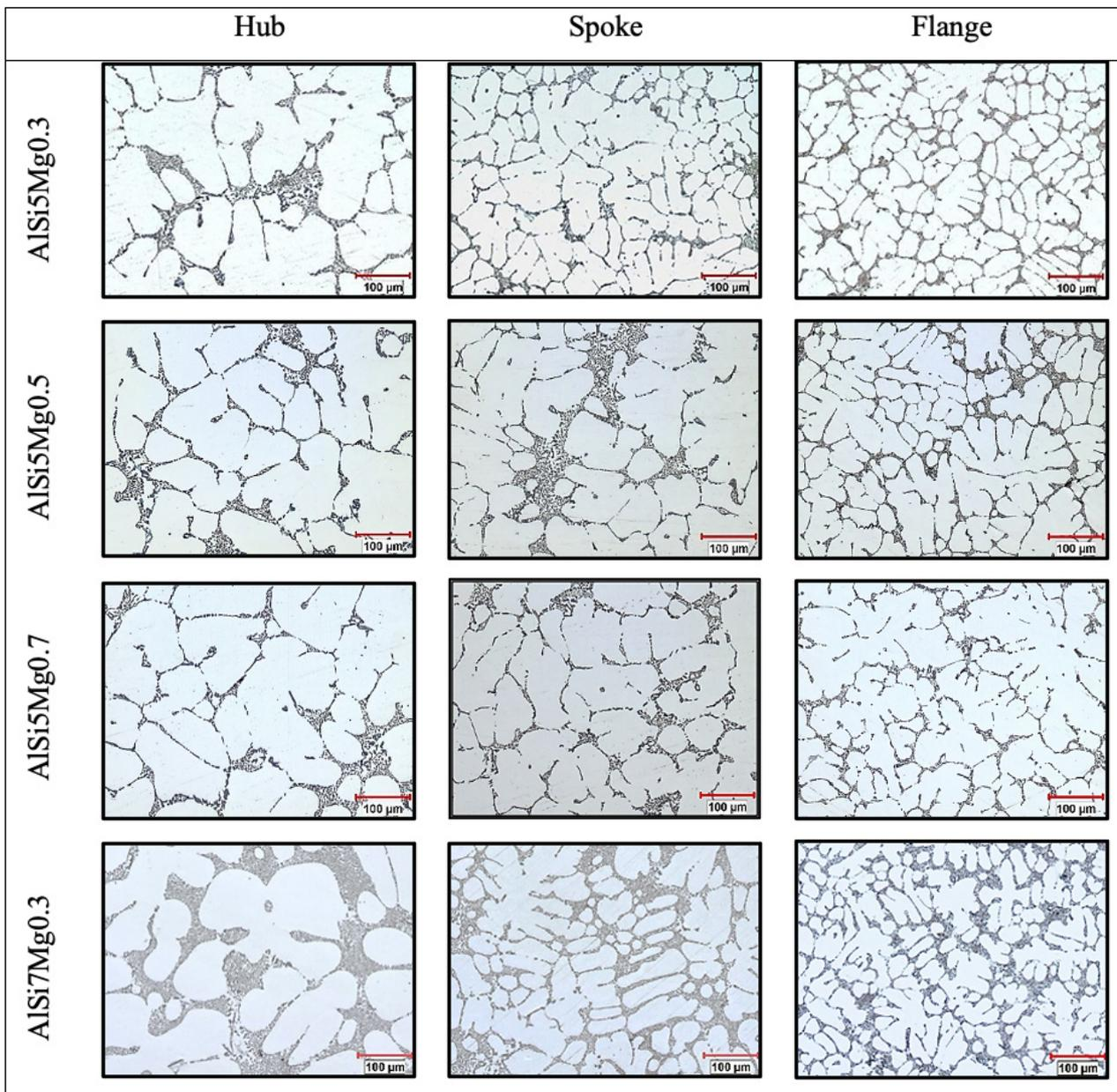
FIGURE 7. Optical microscope images from different parts of the wheel (200x).
