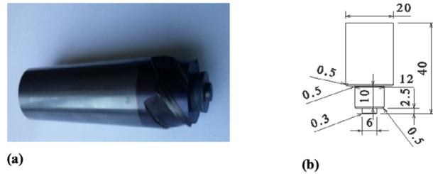
FIGURE 3. a) Photograph of welding tool b) Dimensions of the welding tool (mm).
