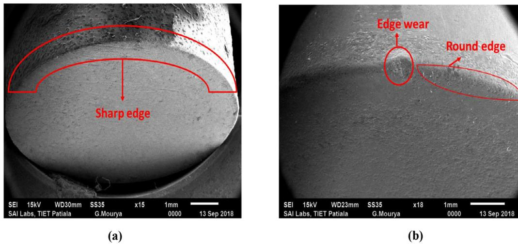
FIGURE 7. SEM micrographs of the tool after machining for (a) expt. N° 9 and (b) expt. N° 2.
