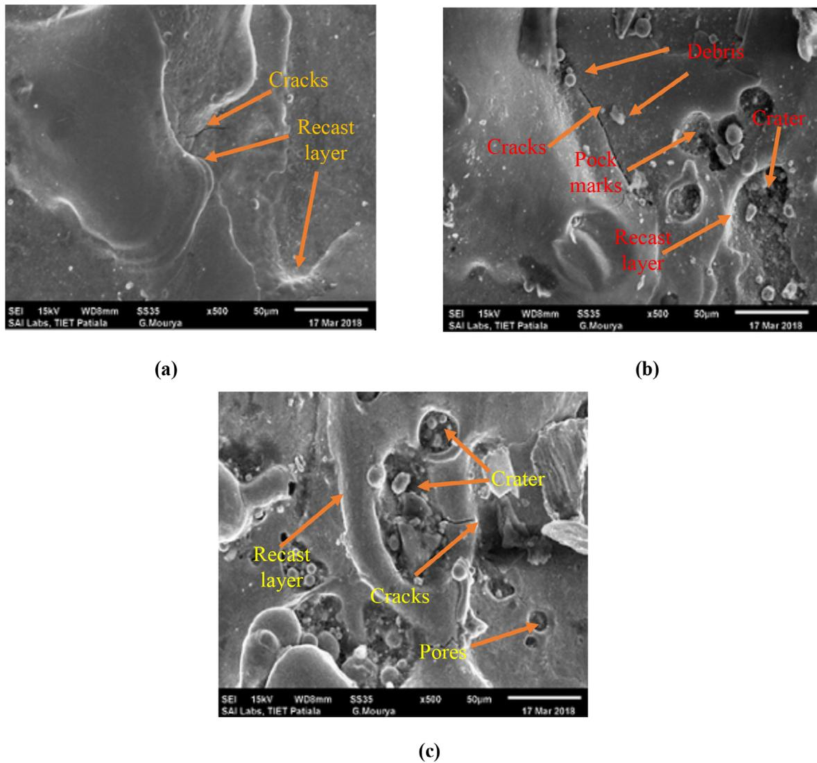
FIGURE 8. SEM micrographs of the tool after machining for (a) expt. N° 9 (b) expt. N° 17 and (c) expt. N° 2.
