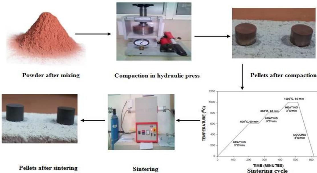
FIGURE 2. Composite tool tip fabrication procedure.
