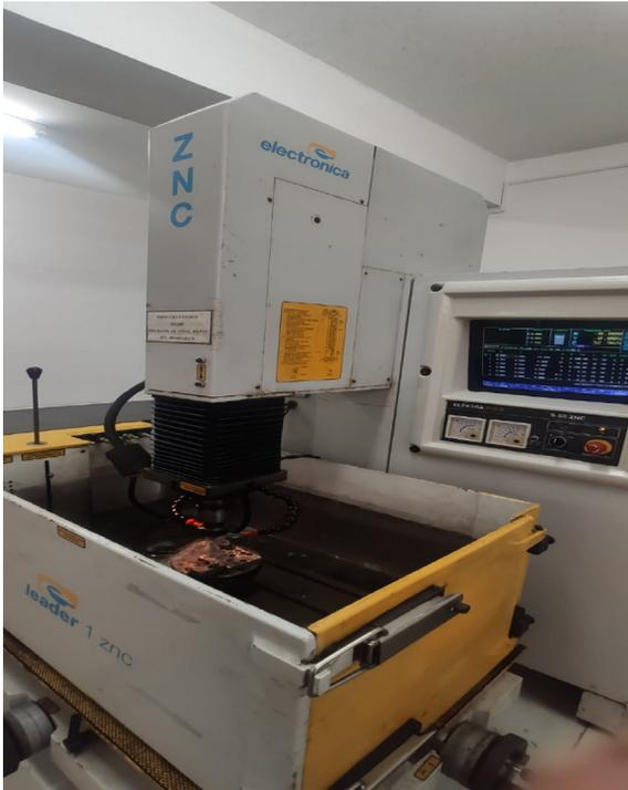
FIGURE 4. Die Sinking EDM machine.
