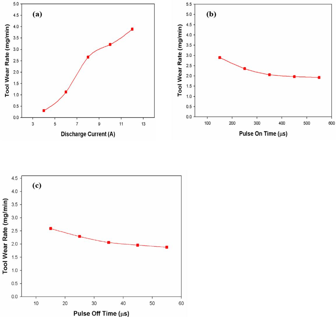
FIGURE 5. Effect of (a)  $I_p$  (b)  $T_{on}$  (c)  $T_{off}$  on the tool wear rate (TWR).
