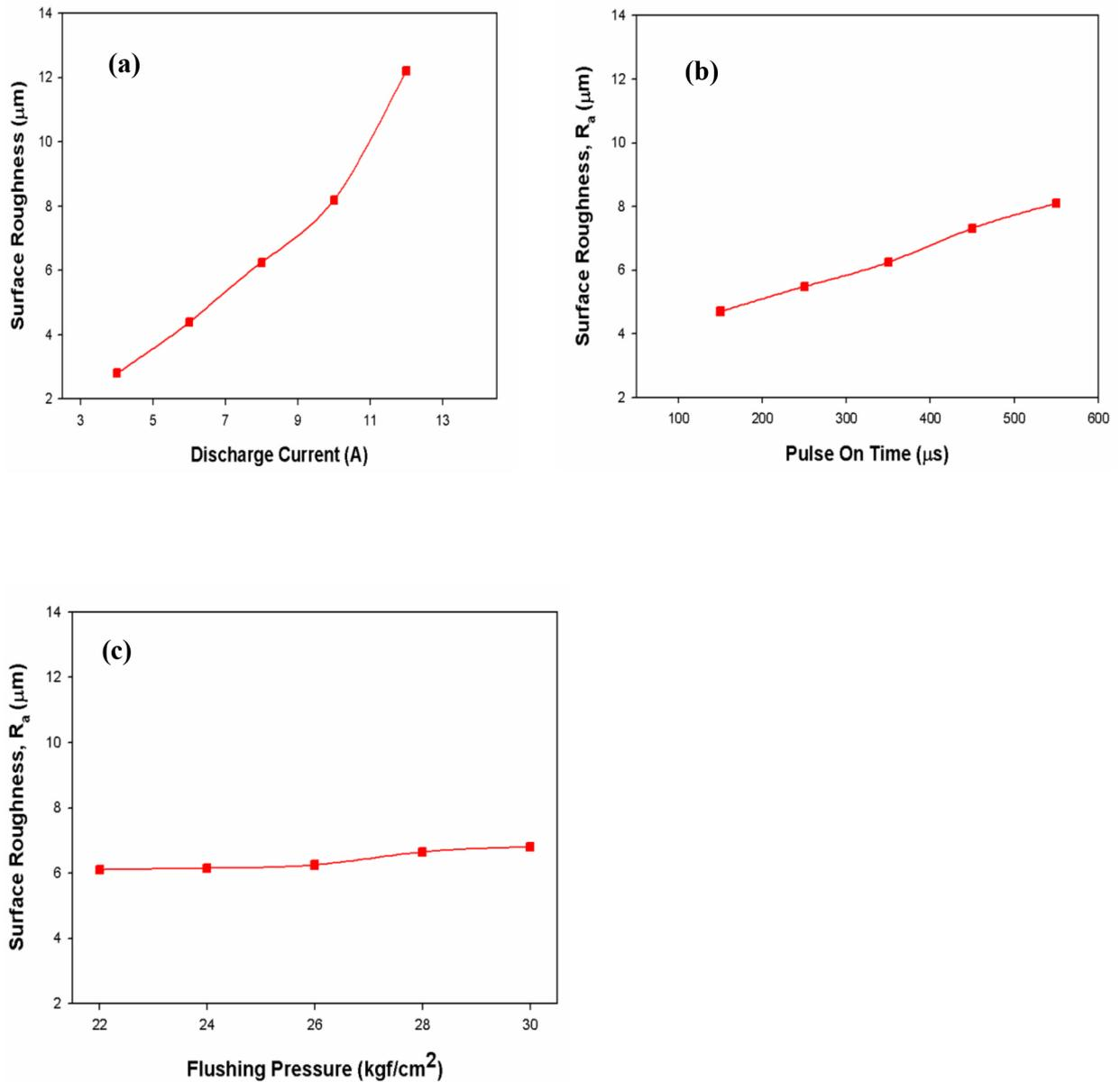
FIGURE 6. Effect of (a)  $I_p$  (b)  $T_{on}$  (c) Flushing pressure on the surface roughness (SR).
