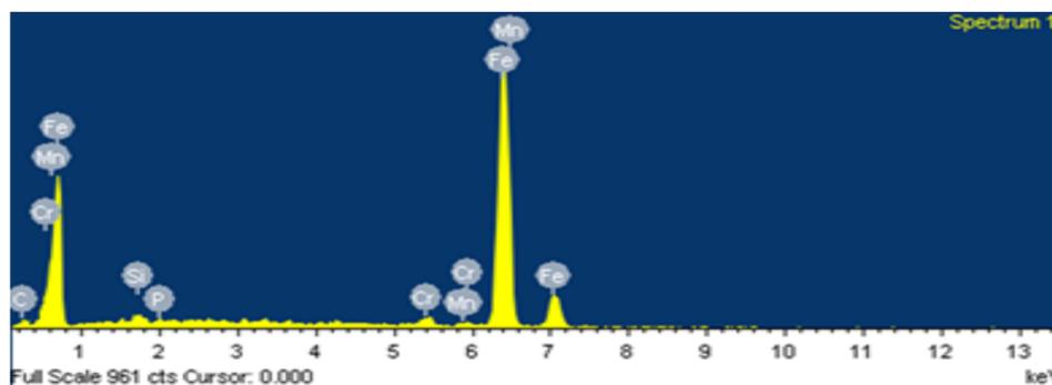
FIGURE 1. EDX of D2 steel.
