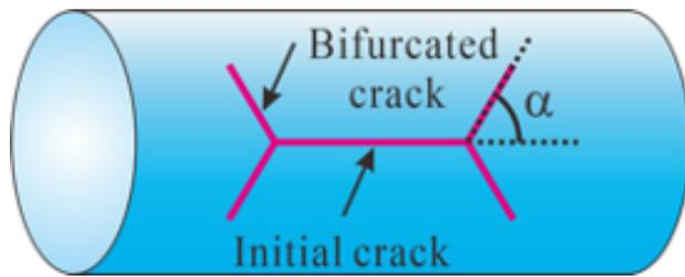
**FIGURE 2.** Schematic illustration of the surface cracking morphologies of CG Cu under cyclic torsional loading with superimposed axial static stress. (a, the angle between the bifurcated crack and the axial direction, is called the measured bifurcation angle.)
