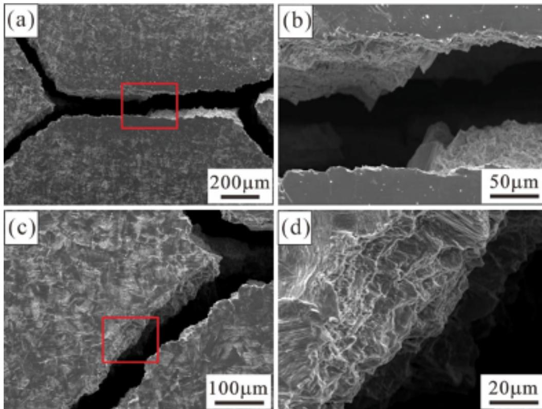
FIGURE 4. Microscopic cracking morphologies of the initial crack and the bifurcated crack on specimen surface of CG Cu under cyclic torsional strain amplitude of 0.61% with superimposed axial static tensile stress of 20 MPa. (a) and (b) the initial crack; (c) and (d) the bifurcated crack; (b) and (d) show the enlarged morphologies in the red squares in (a) and (c), respectively.
