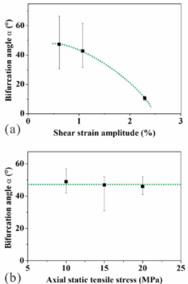
**FIGURE 3.** Statistical result of the measured bifurcation angle,  $\alpha$ . (a) the relationship between  $\alpha$  and the shear strain amplitude when the axial static stress is -10 MPa; (b) the relationship between  $\alpha$  and the axial static tensile stress when the strain amplitude is 0.61%.
