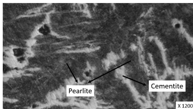
FIGURE 7. Microstructure of iron nugget on optical microscope after etching with 4% Nital.
