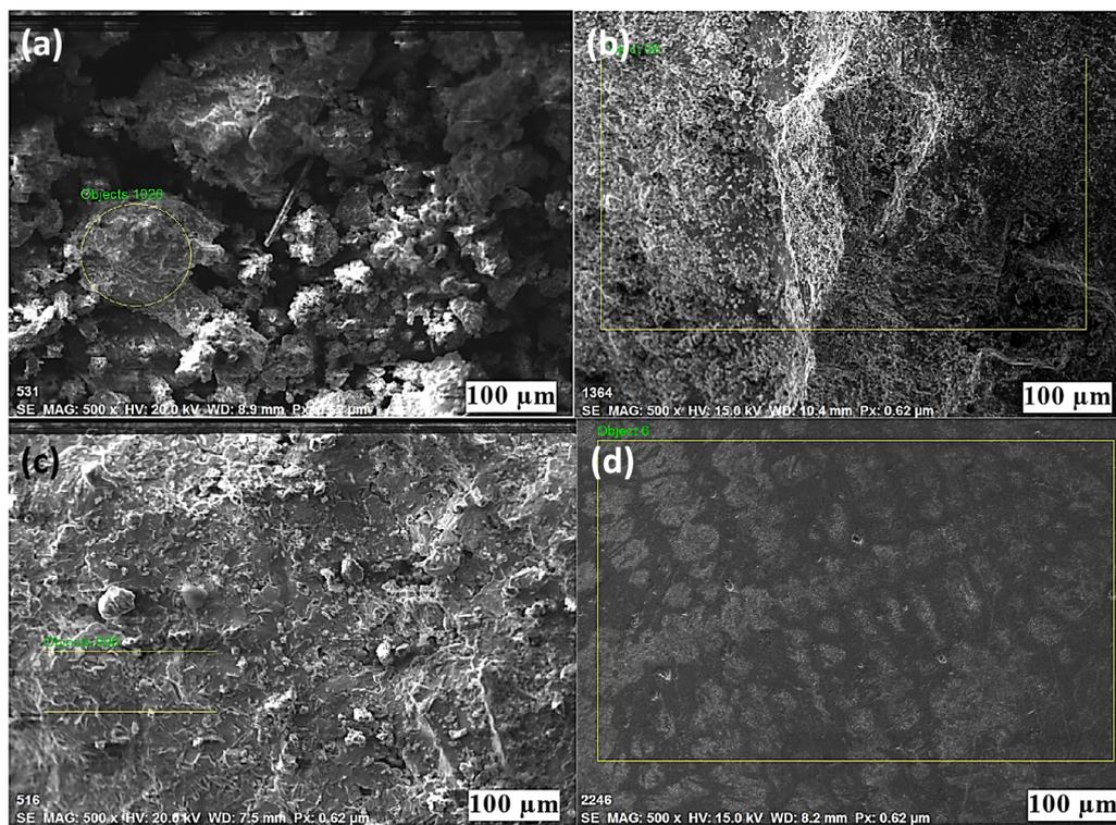
FIGURE 4. SEM image of pellet treated in microwave oven for a. 5 min; b. 10 min; c. 15 min; d. 20 min.
