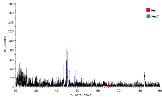
**FIGURE 11.** XRD results showing iron and cementite peaks in microstructure of iron nugget.
