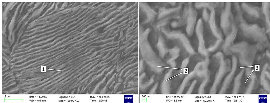
FIGURE 9. SEM microstructure images of the iron nugget. [1] Pearlite; [2] white lamellae are ferrite in lamellar structure; [3] dark areas between white lamellae are cementite.
