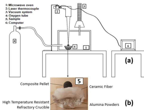
FIGURE 2. a. Experimental apparatus for reduction operations; and b. Design of crucible used in experiments.
