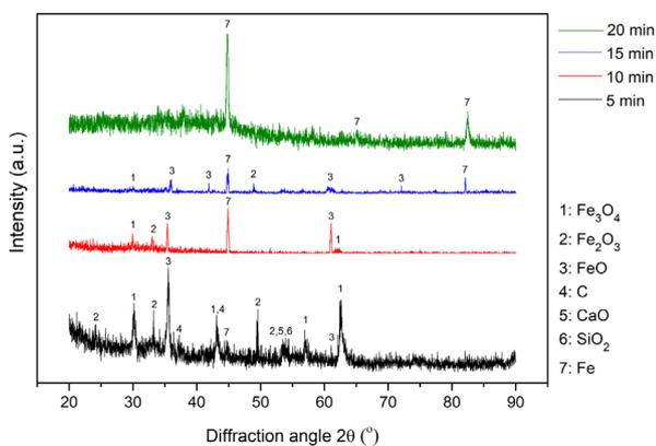
FIGURE 5. XRD patterns of microwave-treated pellets after separation from slag.
