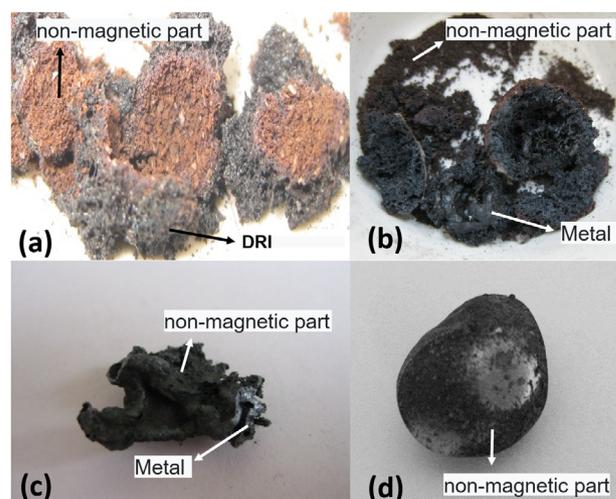
FIGURE 3. Macro image of pellet treated in microwave oven for; a. 5 min; b. 10 min; c. 15 min; d. 20 min.
