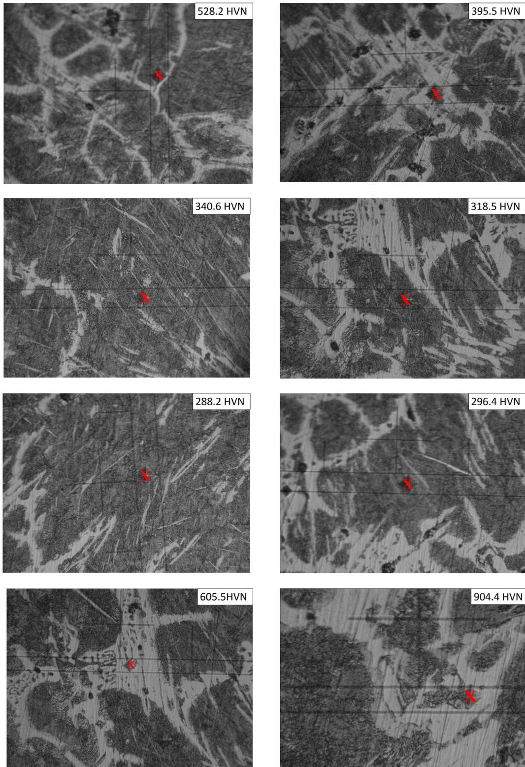
FIGURE 10. Micro-hardness values of phases indicated as "X".
