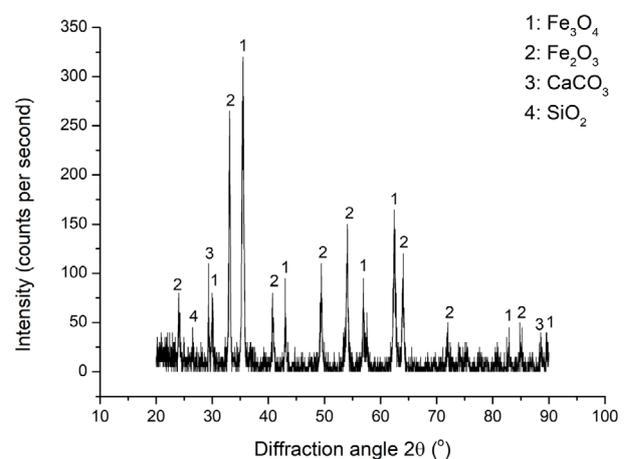
FIGURE 1. XRD image of the concentrate.
