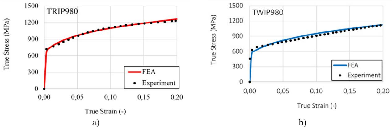
FIGURE 6. The predicted and experimental stress-strain responses for monotonic loading of a) TRIP980, b) TWIP980 steels
