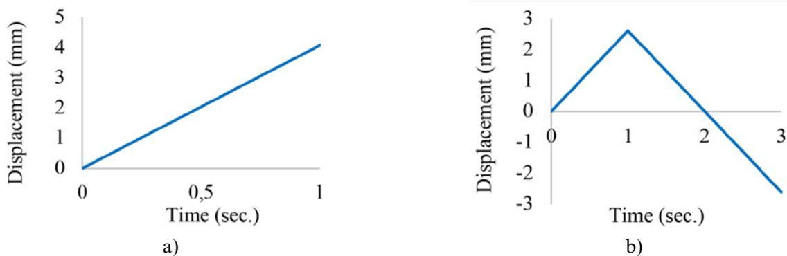
FIGURE 3. Loading history for a) Monotonic, b) Reversal loading
