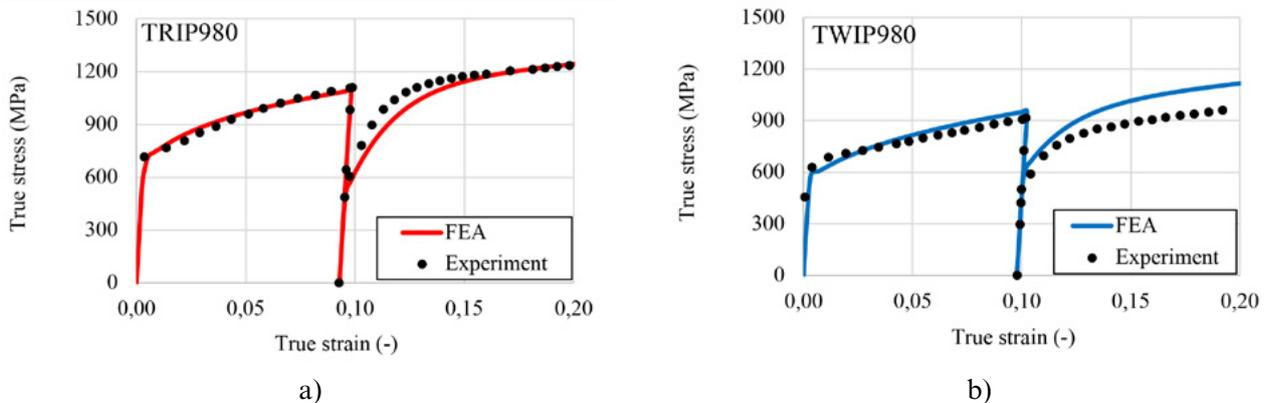
FIGURE 7. The predicted and experimental stress-strain responses for reversal loading of a) TRIP980, b) TWIP980 steels
