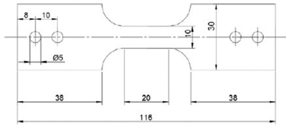
FIGURE 1. Dimensions of test specimen (Joo and Huh, 2018)
