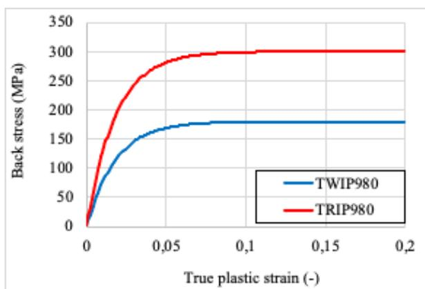
**FIGURE 5.** Back stress curves of the steels
