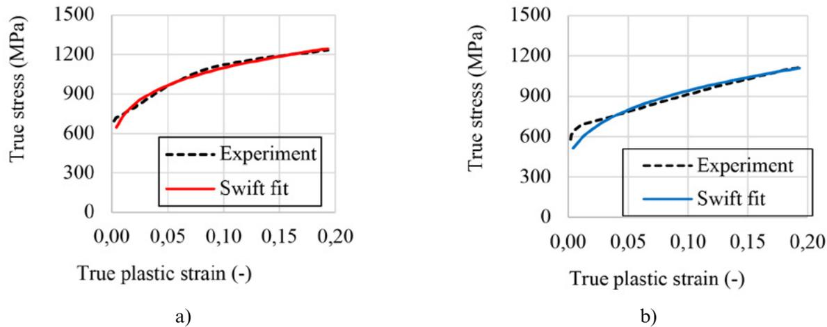
**FIGURE 4.** The hardening curves of a) TRIP980, b) TWIP980
