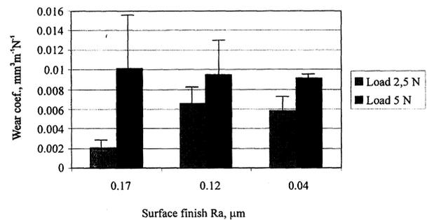
Figure 12. Wear coefficient for different loads and surface finishes
