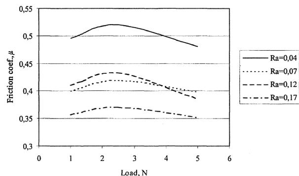
Figure 9. Variation of friction coefficient with load,  $v = 0.15 \text{ m/s}$
