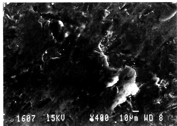
Figure 13. SEM image of the tribofilm and matrix delamination on the pin of Al-VGCF
