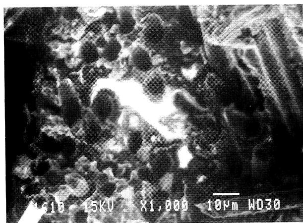
Figure 5. SEM image of Al-exPAN fracture
