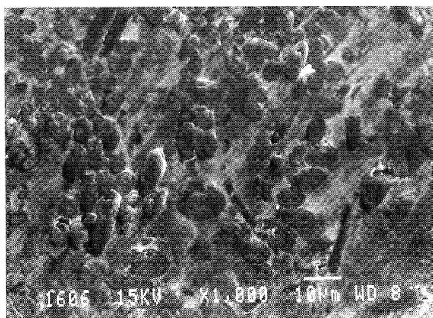
**Figure 14.** SEM image of the tribofilm formed on the pin of Al-VGCF
