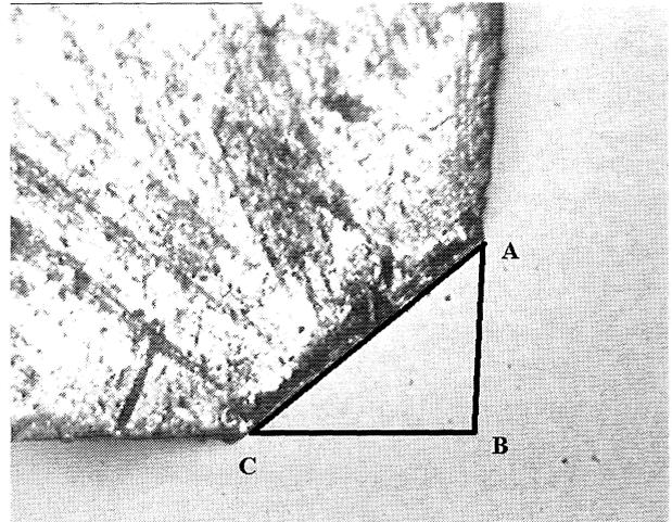
Figure 11. Measurement of wear with image analysis
