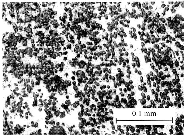
Figure 2. Metallographic image of Al-VGCF
