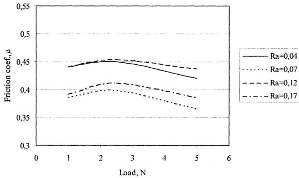
Figure 10. Variation of friction coefficient with load,  $v = 0.30 \text{ m/s}$
