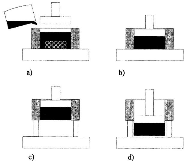
**Figure 1.** Squeeze Casting process: a) Pouring; b) Infiltration; c) and d) Extraction
