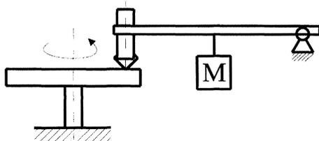
Figure 7. Diagram of tribometer
