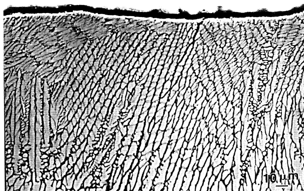
FIG. 7.— Microstructure of Al-Nb alloy after remelting.
