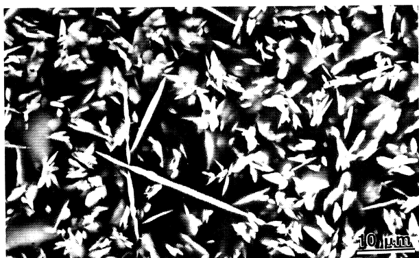
FIG. 6.— Microstructure of remelted layer (R) of Al-Mo alloy.
