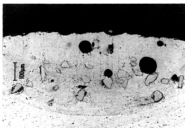
FIG. 1.— Cross-section of Al-Cr alloy produced by LSA.
